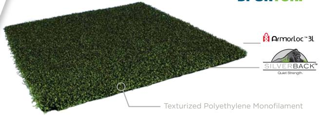
**PROPERTY DESCRIPTION Primary Yarn Polymer** Polyethylene Yarn Cross Section Texturized Polyethylene Monofilament Field Green Standard Color White; Yellow Additional Colors Available **UV Stabilized** Tufted **Fabric Construction** ArmorLoc™ 3L dual layer polypropylene **Primary Backing** SilverBack™ Polyurethane **Coating Type** Yes Perforations 6000/8 Texturized Polyethylene Denier/Ends 1-2 lb. Silica Sand per sq. ft. optional **Recommended Infill** 7/16" **Pile Height** 48.07
